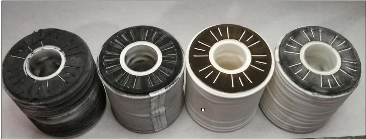
Filters in various stages of contamination
