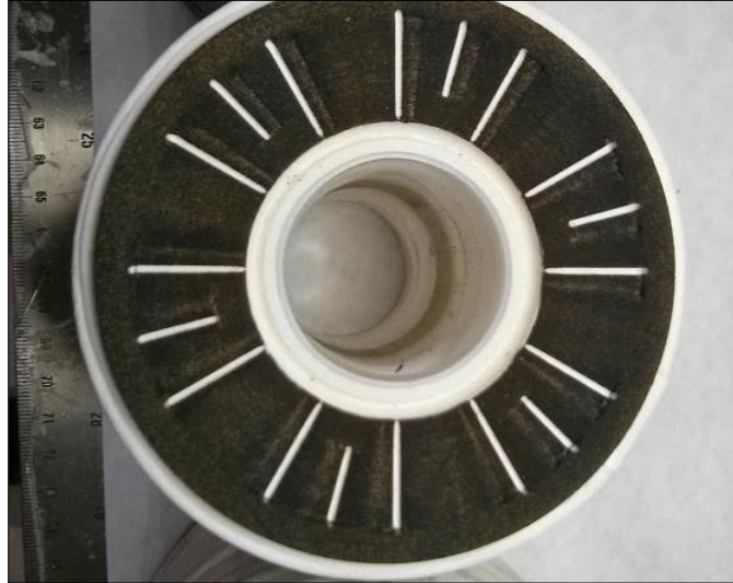
Filter "Dirty Natural Gas"
