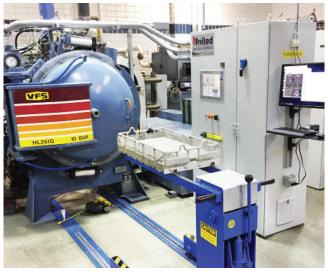
Vacuum furnaces after completion of upgrade, encompassing new control systems with a Protherm 710 process controller to boost operational efficiency and connectivity to the Protherm 9800 Scada application for greater visibility of operations.
