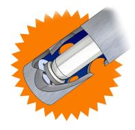
The AccuCarb LTA is an oxygen sensor designed specifically for annealing atmospheres and temperatures. While the electrode designs of standard oxygen probes fall short due to the high impedance of the device at annealing temperatures, the unique electrode contact and solid electrolyte substrate of the AccuCarb LTA takes care of this problem. The sensor is also gas-tight for hydrogen applications to ensure safe operation.
