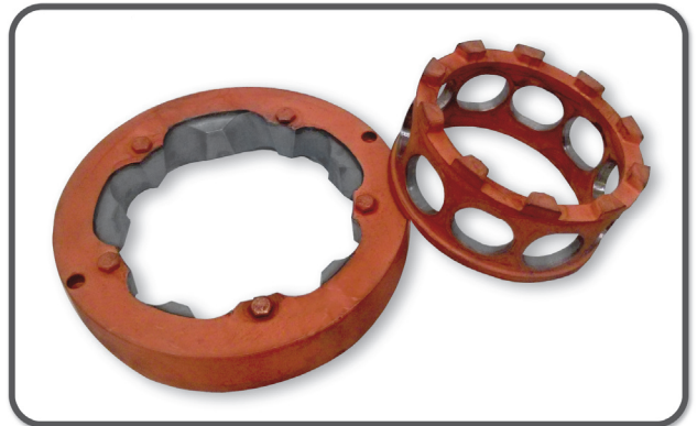
AMS 2418 Type 2 copper plating stop-off on part
