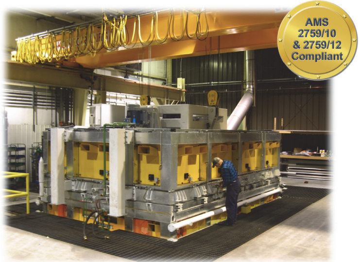
Furnace has a cuboid work zone measuring 17' x 8.5' x 7' and can run loads weighing up to 55,000 lbs.
