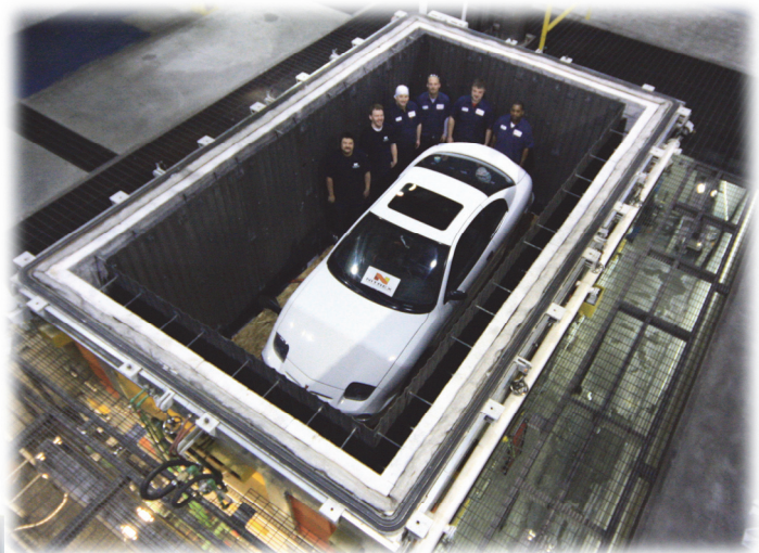
Furnace has a cuboid work zone measuring 17' x 8.5' x 7' and can run loads weighing up to 55,000 lbs.
