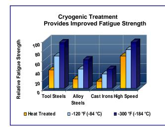
After vacuum treatment it is frequently desirable to subject the work piece to a cryogenic treatment. This process induces carbide particles to precipitate into voids in the iron lattice, thus creating a denser, more stabilized structure that reduces friction, wear and thermal softening. In summary the process:
