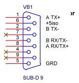
The shield has to be connected with the plug-case.
