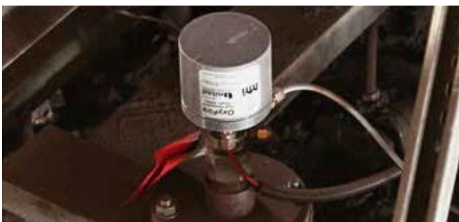
Oxyfire™ In-Situ Zirconia Oxygen Sensor is designed to measure excess oxygen in combustion processes
