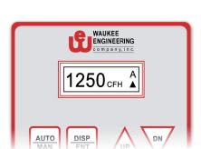
LCD display provides easy-to-read indication of operation values, parameters and faults. Valve-Tronic Plus™ measures and controls the actual flow rate in engineering units.
