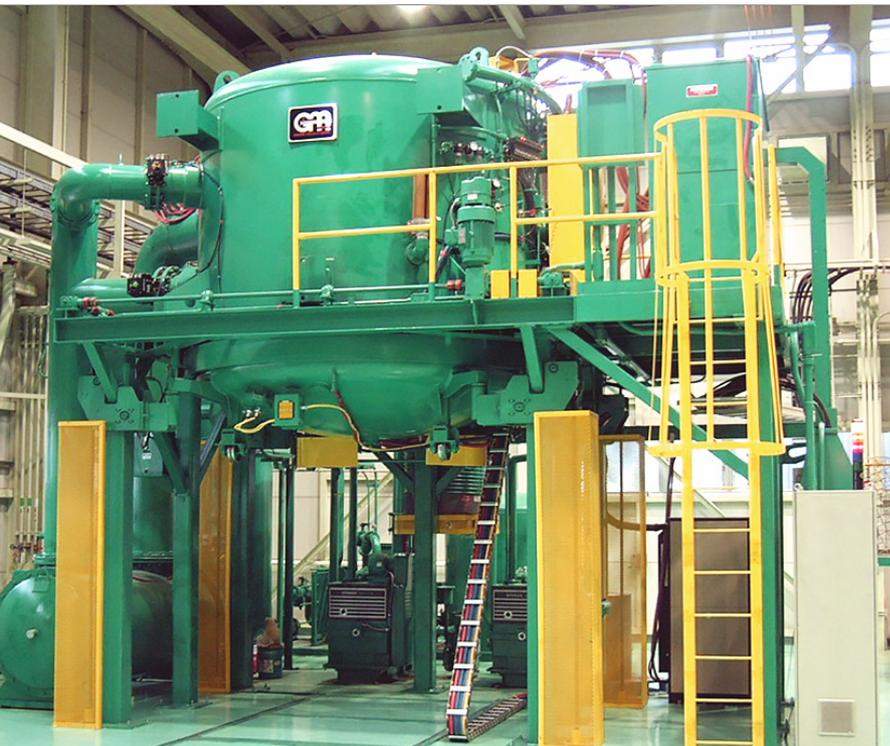
The Vertical Vacuum Furnace series is designed for bottom loading applications and utilizes a circular design hot zone that provides for taller and larger workloads. With the hot zone having gas cooling nozzles 360° around the workload, combined with an external gas recirculation blower and fin/tube heat exchanger, the cooling gas is evenly distributed throughout the work area and optimum cooling is achieved.
