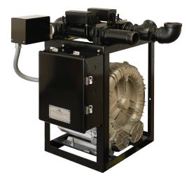
The EndoInjector $^{\text{\tiny TM}}$  is a precision gas mixing and control system for endothermic gas generators. The system incorporates a patented fuel injection design that utilizes electronic flow measurement and precise ratio control to consistently provide the ideal gas mixture for highquality endothermic gas generation.
